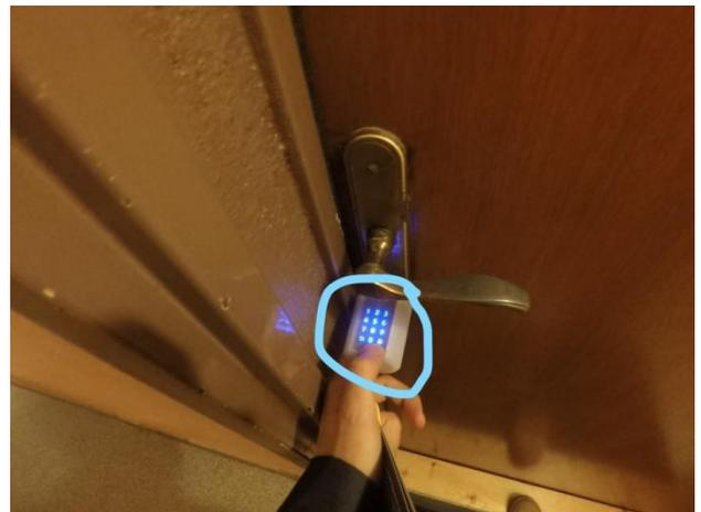
To open the door, push any button to turn on the keyboard
